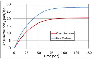
35% increase in angular velocity for 5 m/s wind velocity
