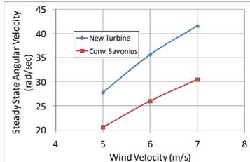
For each wind velocity about 35% increase in steady state angular velocity
